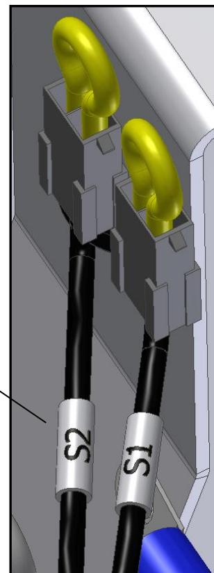
Connect extension cord to the cord marked S2 and fasten it with cable binders as shown.
