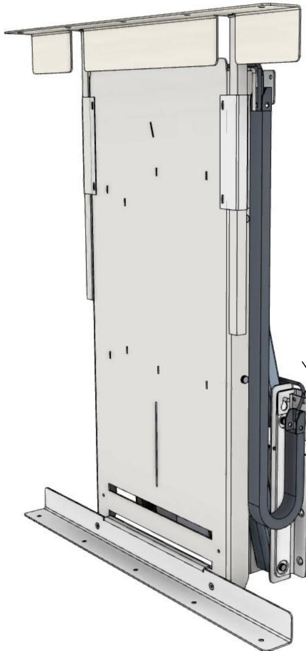
Loosen the nut that keeps the cable track in place, pull cable track aside
