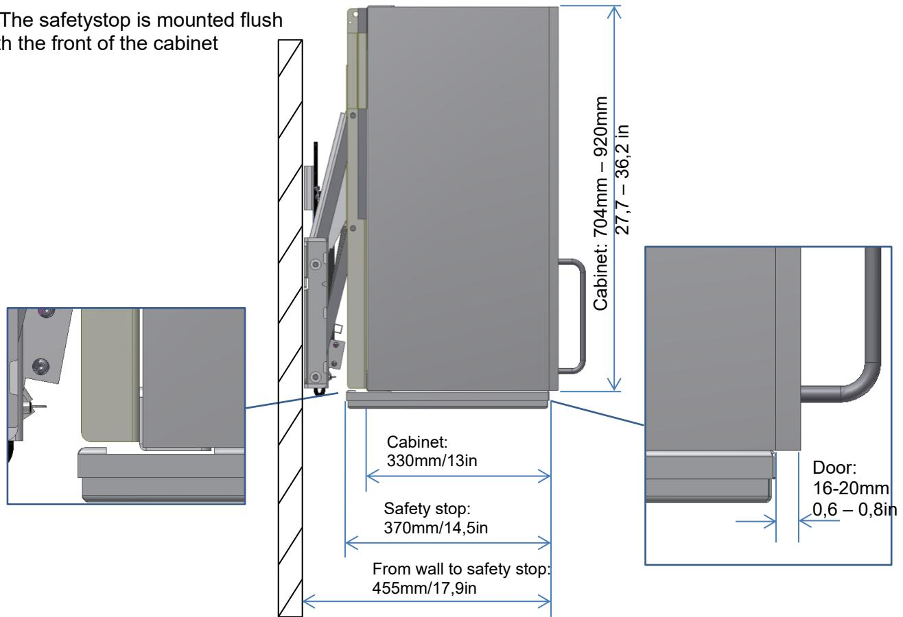
2: The safety stop is mounted flush with the front of the cabinet door
