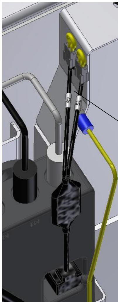
Remove yellow 2,2k $\Omega$  resistor from the cord marked S2
