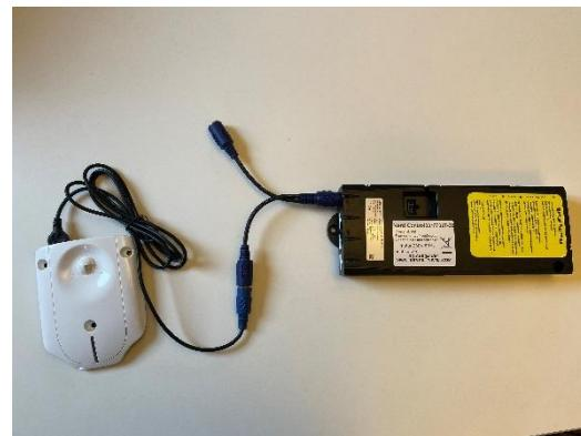
6.7.2 Insert the split-cable in the plug "HS" in the control box. Then, insert the adapter in one end of the split cable, and the button that came with the product, in the other
