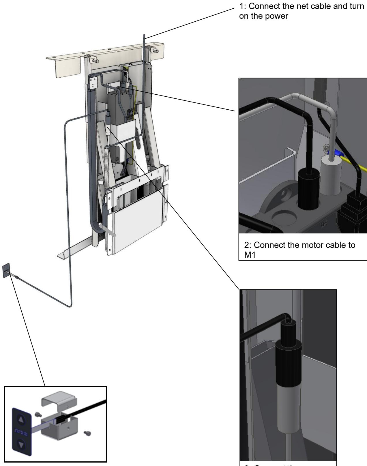
When the handswitch is placed at the desired position, Cable support for control switch can be mounted
