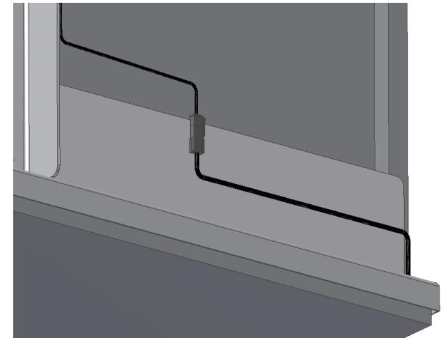
Place plug with yellow 2,2kΩ resistor on the right side of safety stop plate (shown from the front)
