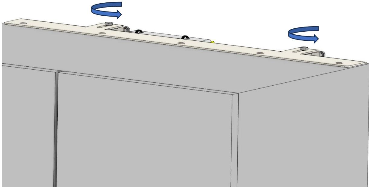
2. Adjust the leveling screws from behind the unit
